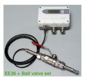
$a_w$  = 0 corresponds to water-free oil, while  $a_w$  = 1 describes fully saturated oil.  $a_w$  measurement with EE36 transmitter series is based on the outstanding long term stability and resistance to pollution of the E+E capacitive sensor elements series HC.
