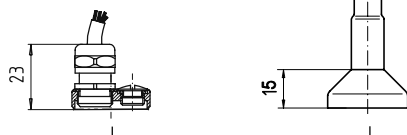
flying lead with access to zero and span pots, IP 68
