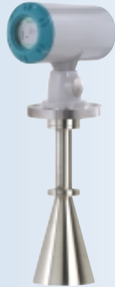
Horn with waveguide extension. Used for high temperature isolation, long nozzles, and clearing tank obstructions.
