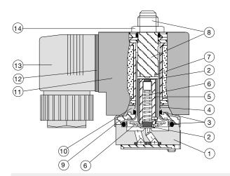
Valve body: **Brass** 2 Plunger seal: FPM (Viton)
