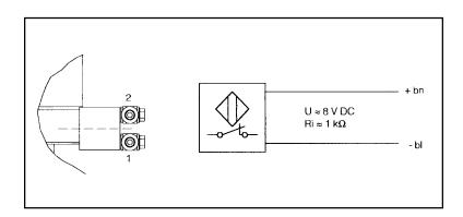
The lower limit switches are always used for the "Measurement" function, the upper swithces for the "Maintenance" function.
