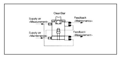
The CleanStar A935 Retractable Housing is operated with an air pressure of 4 to 6 bar (58 to 87 psi). The air must be filtered (40  $\mu$ m) and free from water and oil. There is no continuous pressure demand. The air lines must have a minimum nominal diameter of 4 mm for the pneumatic postion Indicators.
