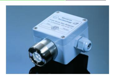
The T100 is a 4-20mA 2-wire transmitter can measure a wide range of gases and is housed in a rugged, compact metallic enclosure. It incorporates advanced SMD electronics and a 3 electrode electrochemical sensor based on micro fuel cell technology, designed to be maintenance free and inherently stable.
