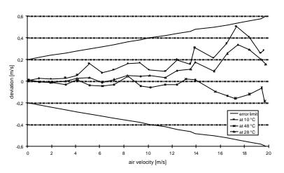
Due to the mass flow measurement principle, the accuracy is highly dependent on the temperature.
