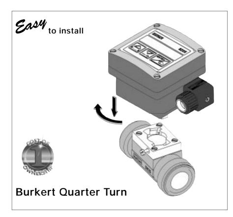
The recommended In- and Outflow straight pipe length should respect 10xD in and 3xD out. According to pipe's design, necessary distances can be bigger or use a flow conditioner to obtain the best accuracy. For more informations, please refer to EN ISO 5167-1.
