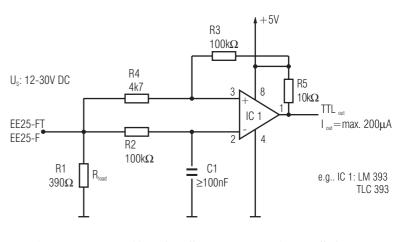
Using a comperator with push-pull output stage R5 is cancelled!
